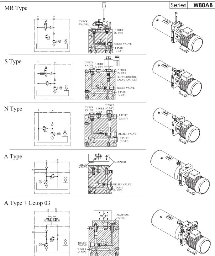
The W80AB power pack series is designed for use with European standard B14 AC motors.
